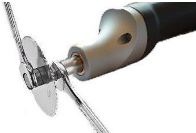
Fig. 1: Releasing the retaining screw
